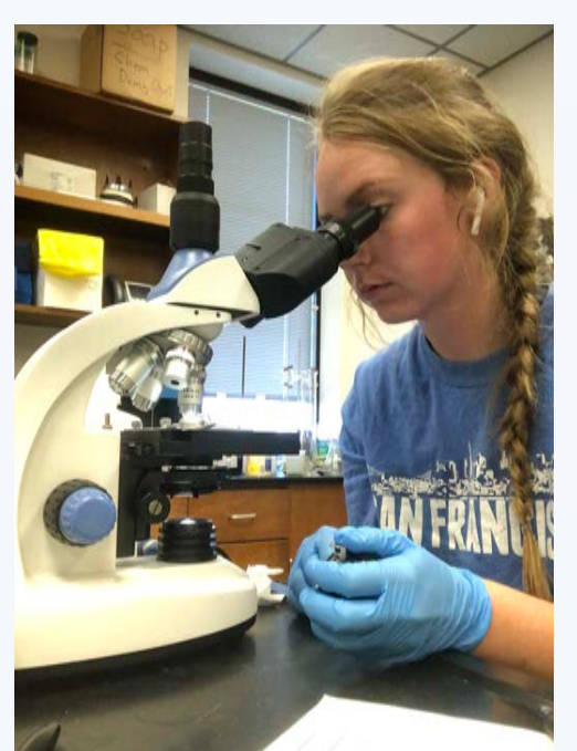
Image 6 depicts the process of counting microplastics using a hemocytometer and microscope.
