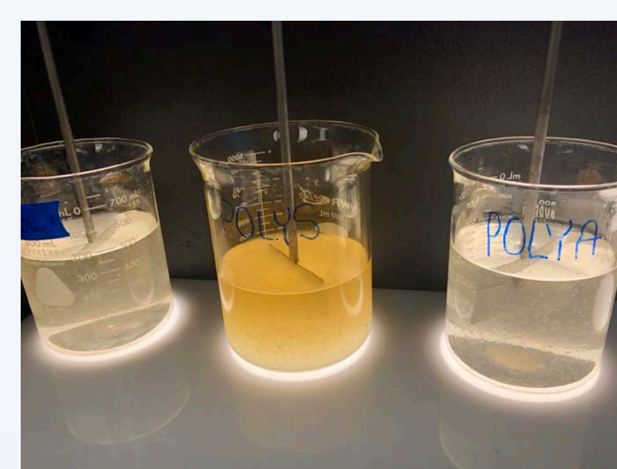
Image 3 displays a Jar test set up using Colorado River Water.
