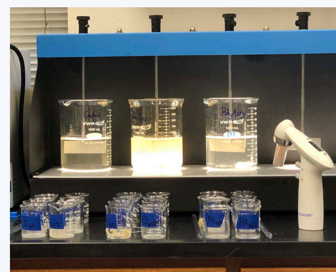
Image 3 displays a Jar test set up using Colorado River Water.
