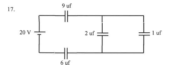
A. What is the total capacitance in the circuit?
