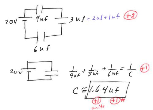
B. What is the charge on the plate of the 6 uf capacitor?
