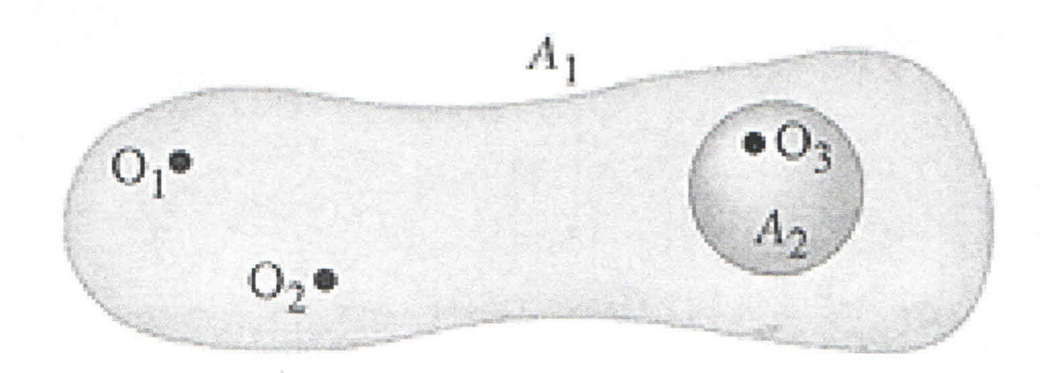
What is the electric flux through the blue sphere A<sub>2</sub> of radius 10 cm?
