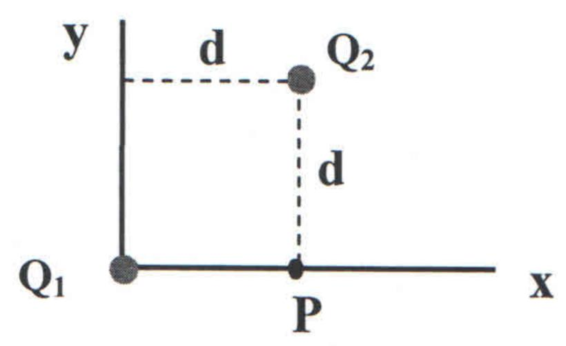
Find the electric field at point P on the x-axis.
