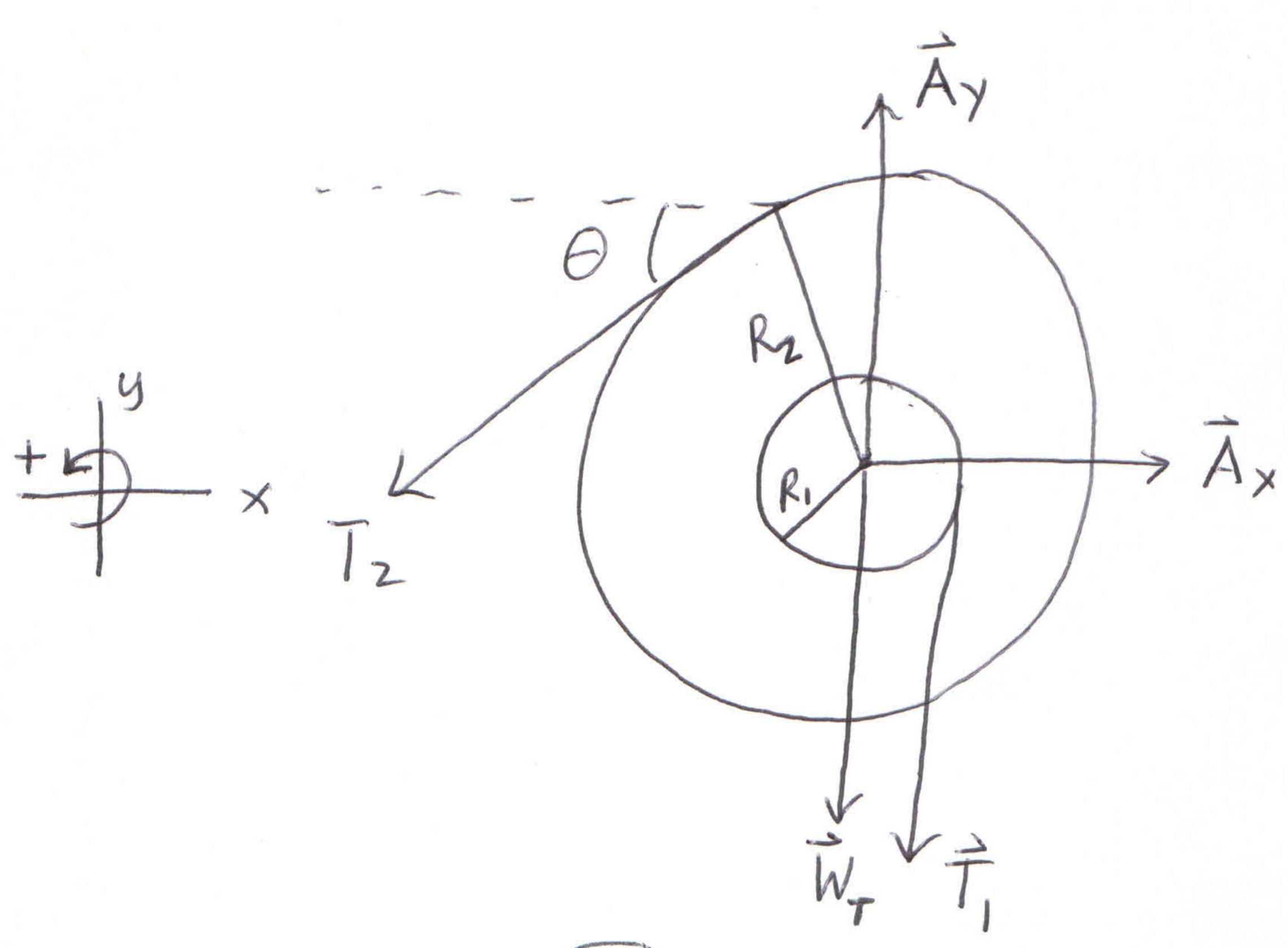
5 forces D+1/2 each = 2.5 3 anglest dimensions @1/2 = +1.5 Body is I solated = +D 1 Axis with Rotation = +D
