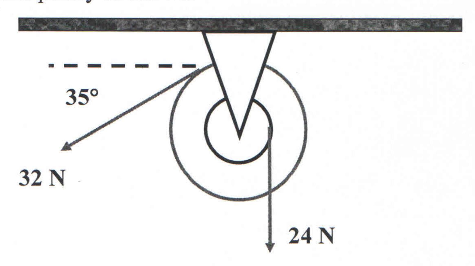
6 pts A. Draw a proper Free Body Diagram of the compound pulley.
