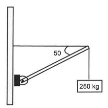
**A.** Draw complete free body diagrams for both the 250 kg block and the beam.
