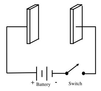
Since there is no net charge on either plate, there is no electric field between the plates and no electric potential energy stored.
