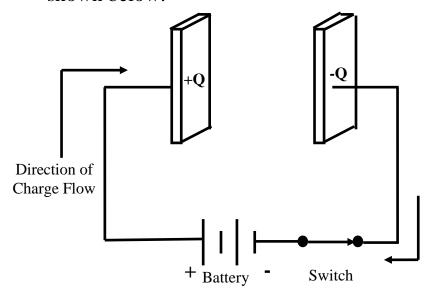
The <u>separation of charge</u> produces an electric field  $\underline{\vec{E}}$  between the plates. Thus, an electric potential difference exists across the plate and electric potential energy is stored in the system equal to work done by the battery in transferring the charge between the plates.
