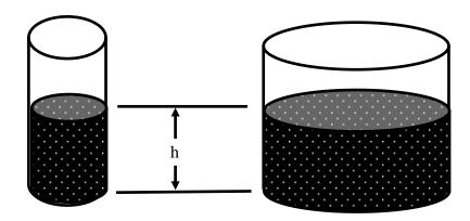
In our diagram, it is easy to see that the wider glass (largest area) contains more water when the <u>water</u> in both glasses is <u>at the same height</u>. By analogy, a capacitor whose conductor has a larger surface area can hold more <u>charge</u> for a given electric potential difference.
