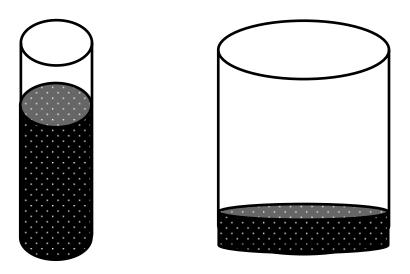
A smaller capacitor has a greater voltage for the same charge just as the water will have a greater depth in a smaller capacity water tank for the same amount of water.
