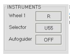
Press the Wheel or Selector buttons to bring up (forward) the <u>Auxiliary (Installed) Equipment</u> tabbed dialogue in which options for the filter wheel or port selector can be managed. The Autoguider button will bring up (forward) the autoguider control panel:
