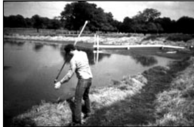
Figure 2. Lagoon effluent samples being collected with a bottle attached to a pole extension.
